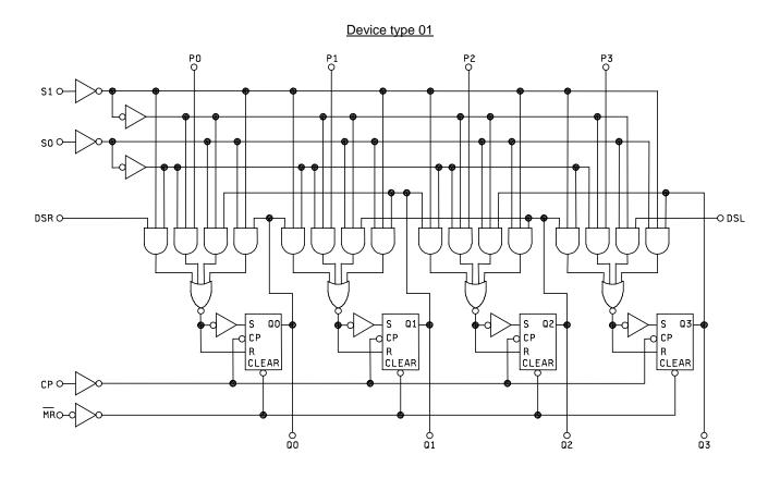
FIGURE 2. Logic diagram.
