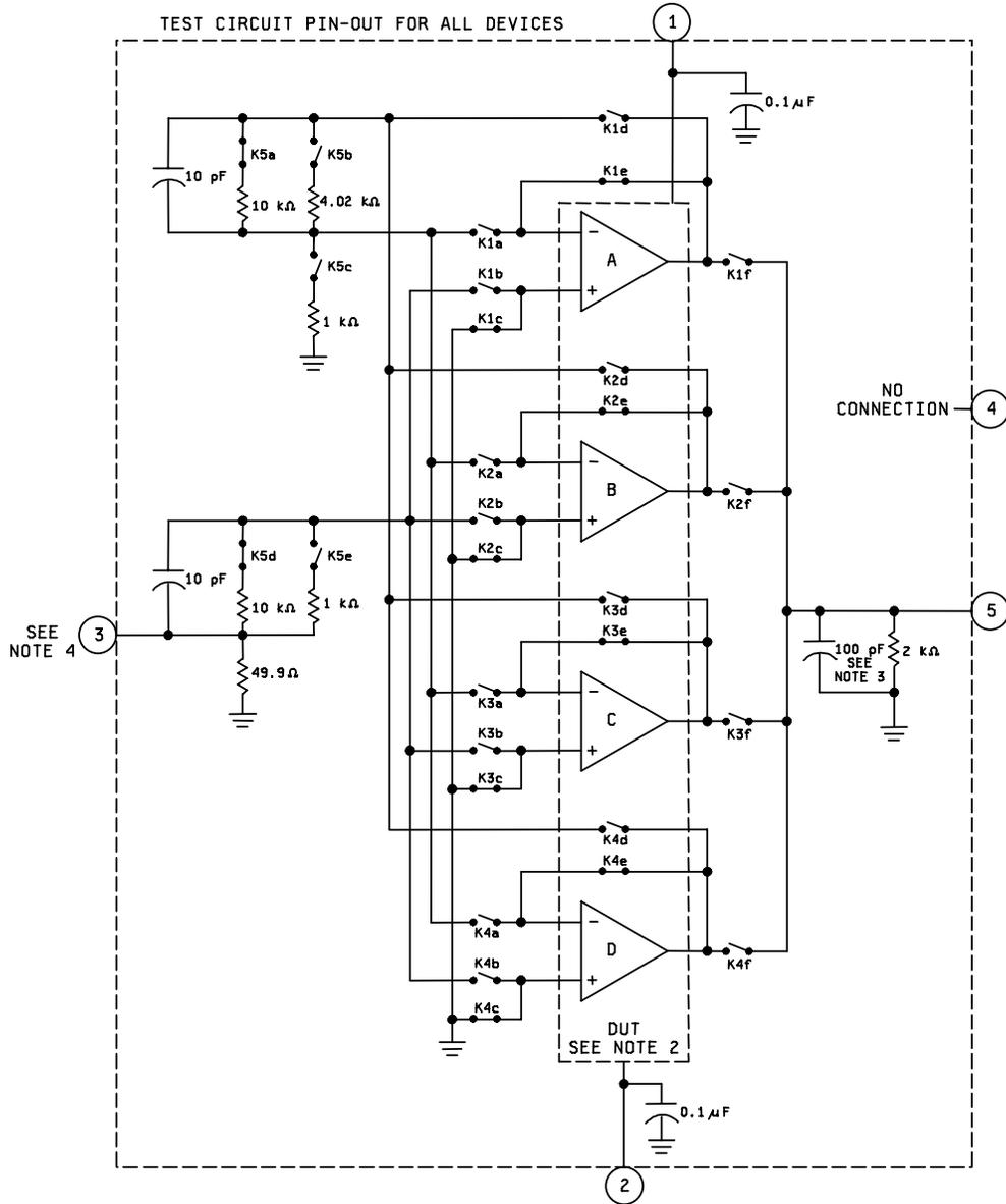
FIGURE 4. Test circuit and waveform for transient response .
