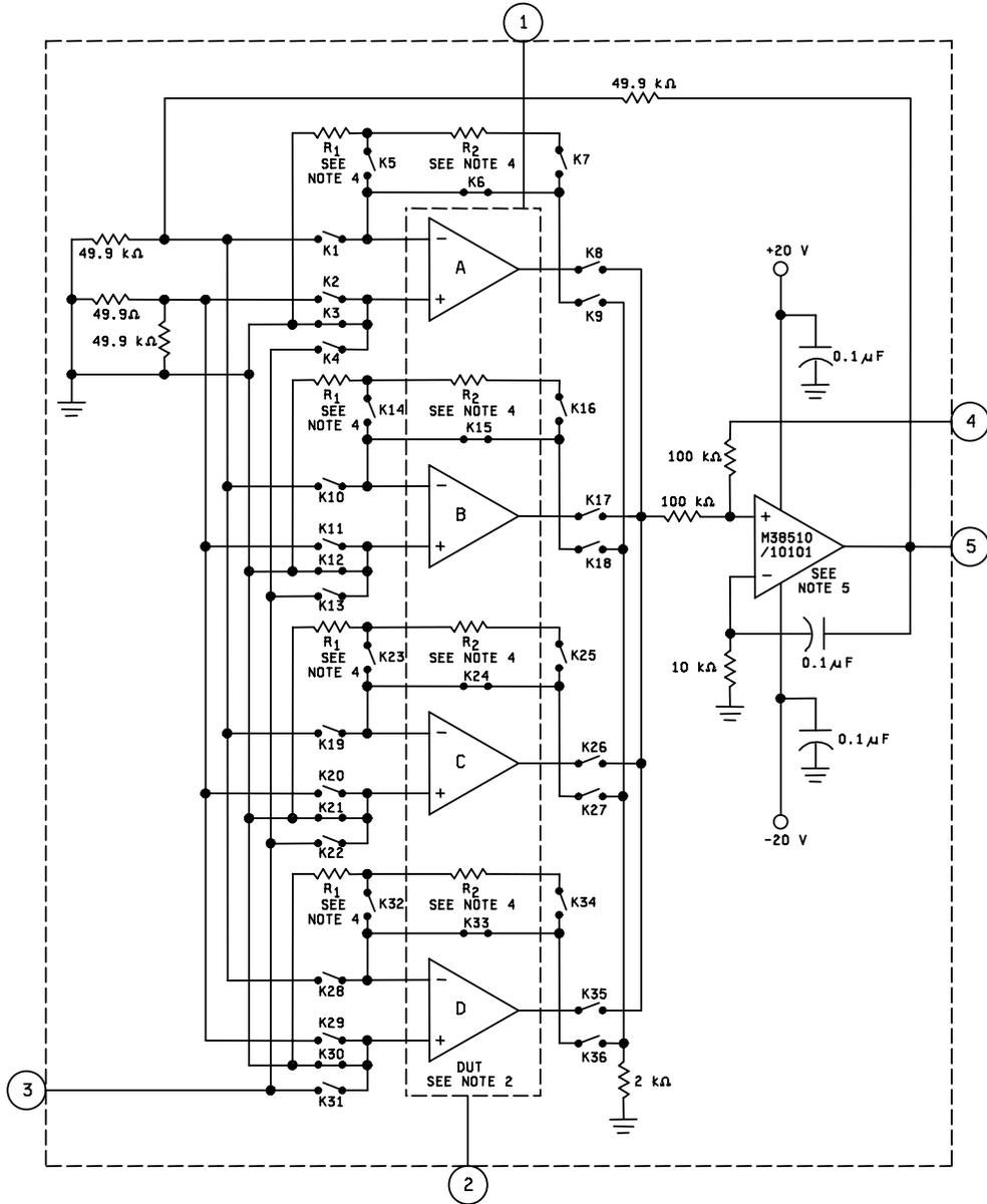
FIGURE 3. Test circuit for channel separation.
