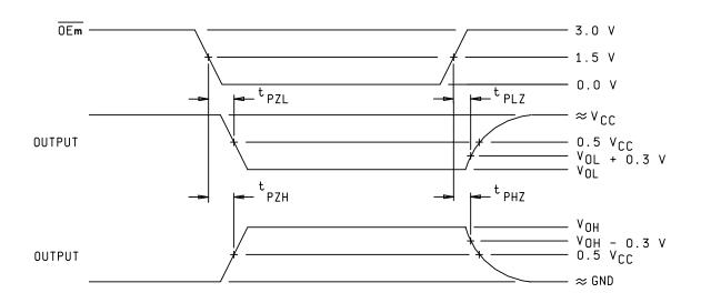
FIGURE 5. Switching waveforms and test circuit.
