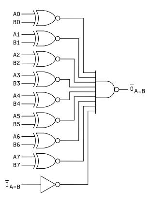
FIGURE 3. Logic diagram.
