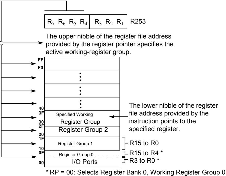
**Figure 12. Register Pointer—Detail**
