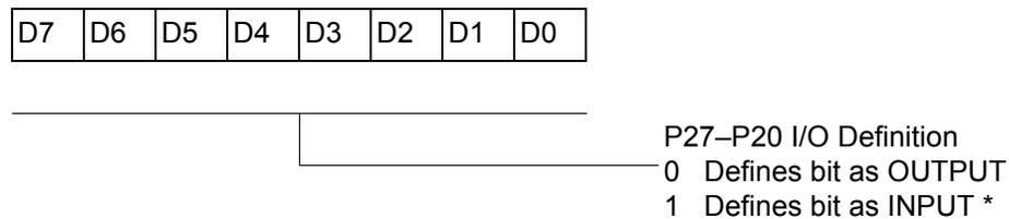
\* Default setting after reset. Not reset with a Stop Mode Recovery.
