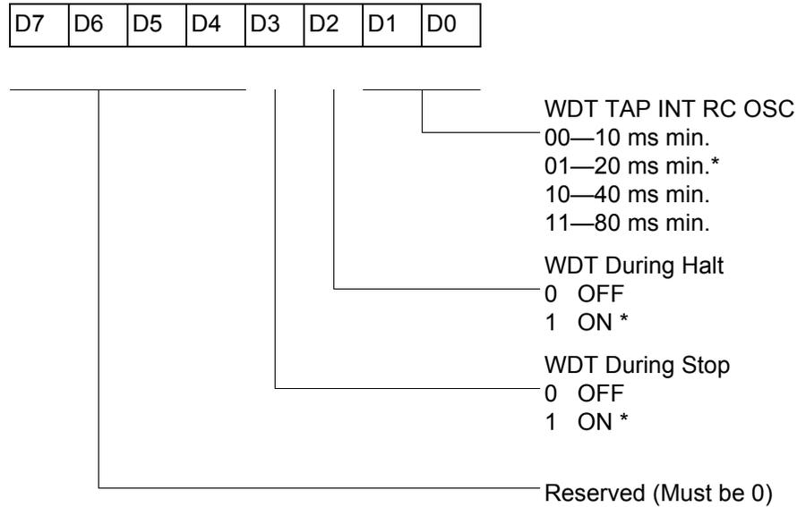
\* Default setting after reset. Not reset with a Stop Mode Recovery.
