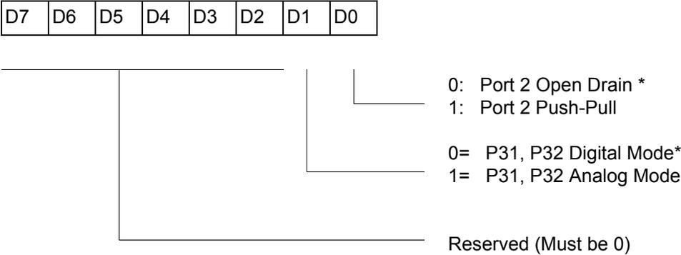
\* Default setting after reset. Not reset with a Stop Mode Recovery.
