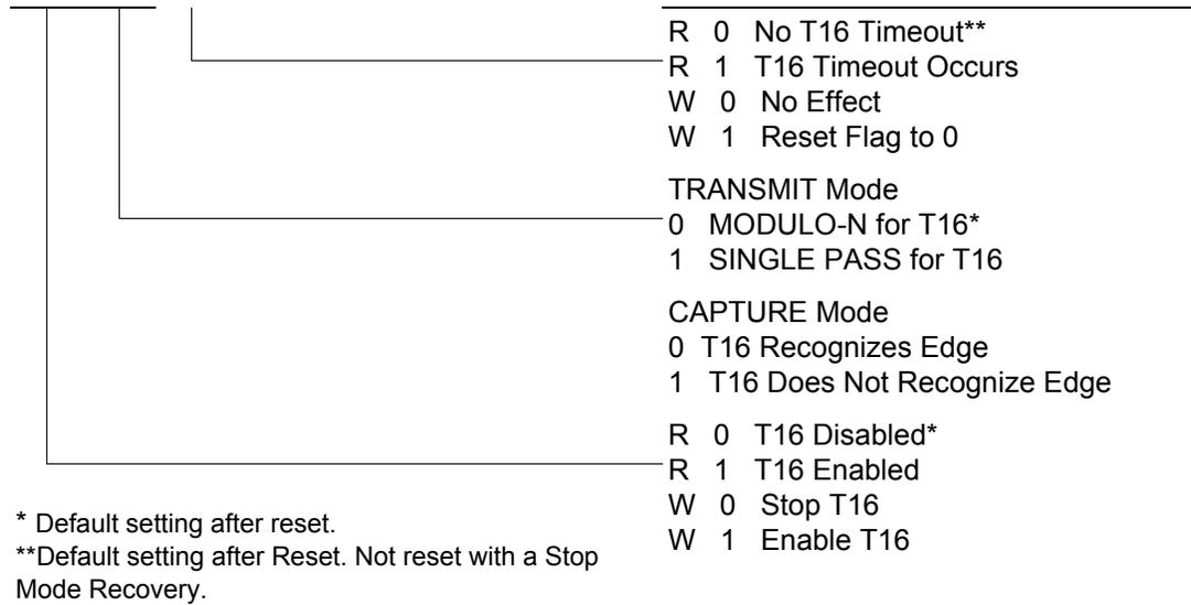
**Figure 36. T16 Control Register ((0D) 02H: Read/Write Except Where Noted)**
