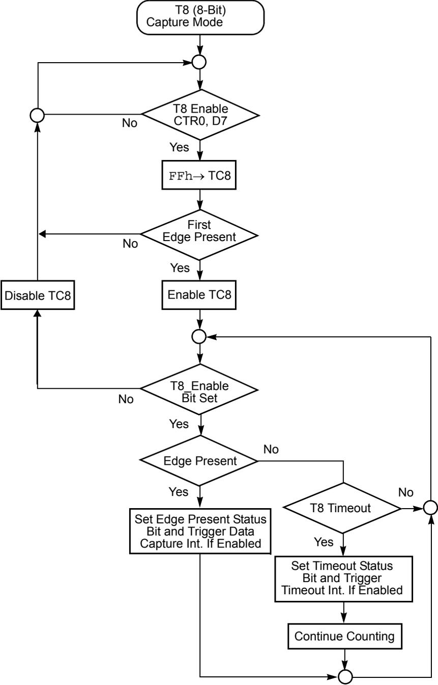
Figure 19. DEMODULATION Mode Flowchart
