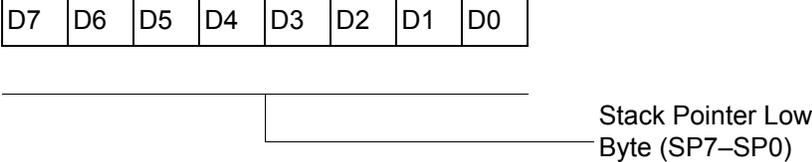
**Figure 52. Stack Pointer Low (FFH: Read/Write)**
