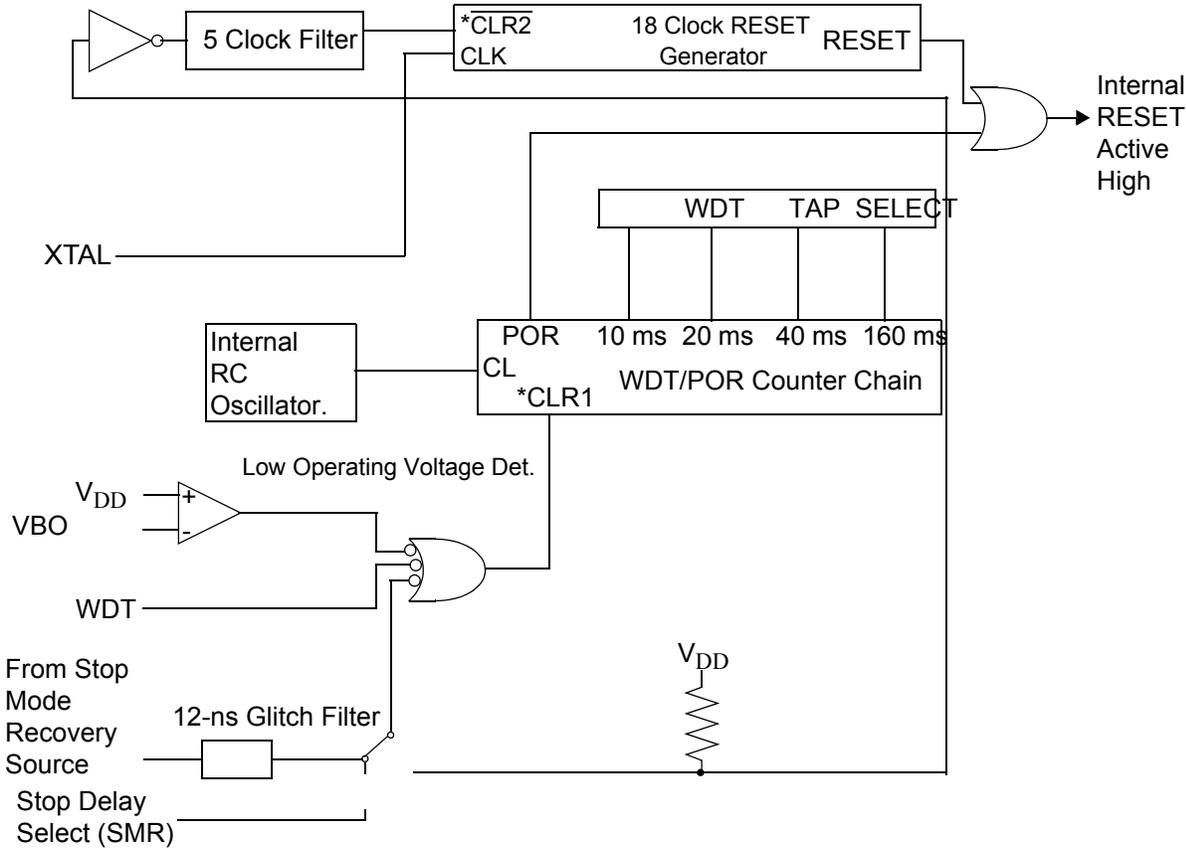
\* CLR1 and  $\overline{CLR2}$  enable the WDT/POR and 18 Clock Reset timers respectively upon a Low-to-High
