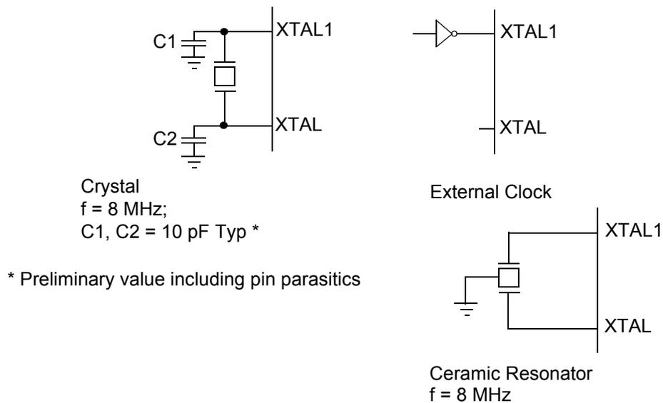
**Figure 26. Oscillator Configuration**
