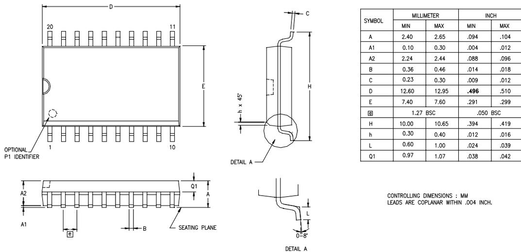
Figure 56. 20-Pin SOIC Package Diagram
