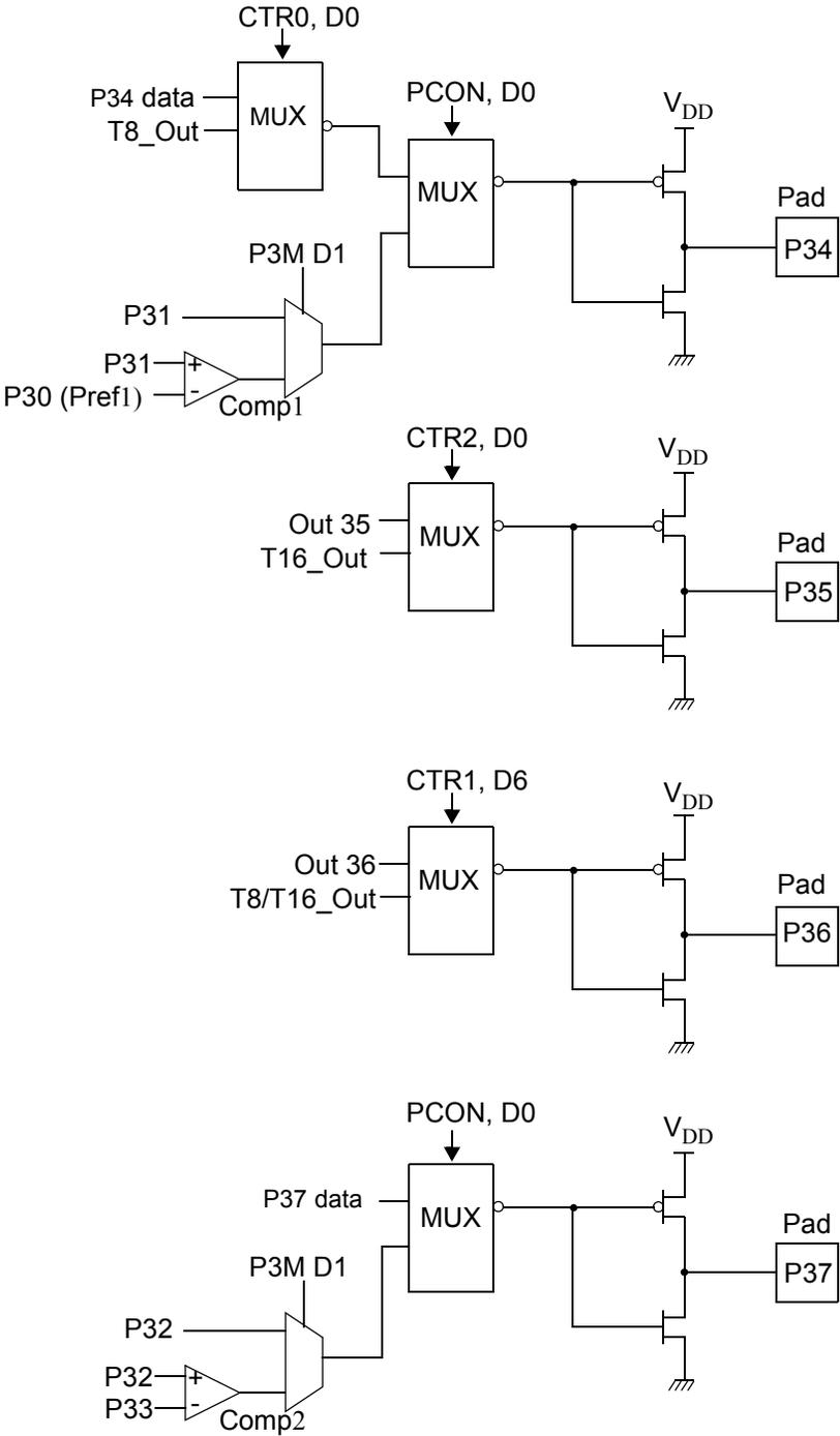
Figure 8. Port 3 Counter/Timer Output Configuration
