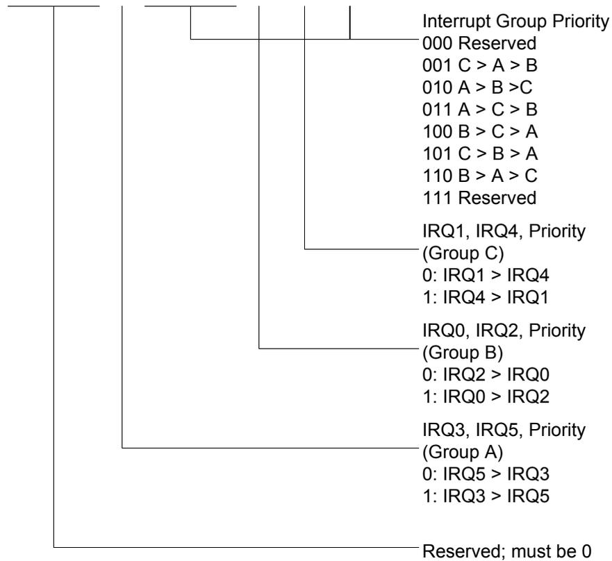
**Figure 46. Interrupt Priority Register (F9H: Write Only)**
