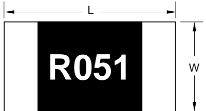
Fig. 5 Chip resistor outlines
