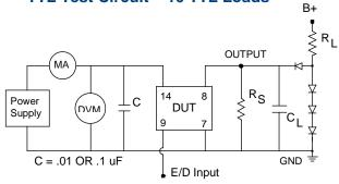
$C_L=20$  PF, Includes Probe Capacitance  $R_L=270$  Ohms;  $R_S=6$  K Ohms All Diodes are 1N4148 or Equivalent
