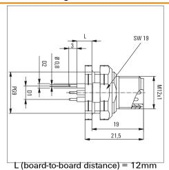
Front panel section D1 = 5.0 mm
