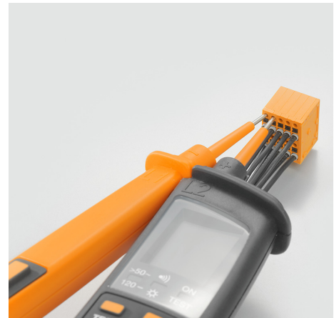
Maintenance through test tap
