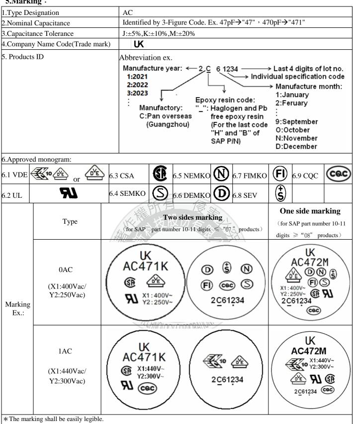
\*"C", Marked with code "\_" stand for Halogen and Pb free epoxy resin.
