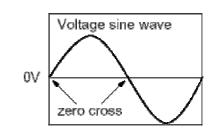
If the test voltage without the raise from near zero voltage would be applied directly to capacitor, the surge voltage may arise, and therefore, the defective may be caused.
