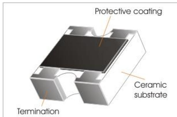
Fig 1. Construction of a Chip-R array (convex Type)
