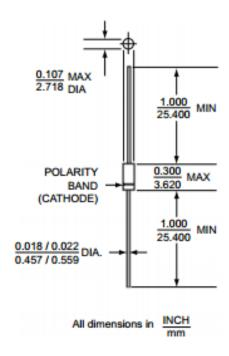
Lead Material: copper clad steel
