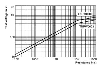
Single-Pulse High Voltage Overload Test 10/700 µs EN 140000 4.27
