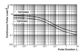
Maximum pulse load, continuous pulses; applicable if  $\bar{P} \leq P \ (\vartheta_{amb})$  and  $\hat{U} \leq \hat{U}_{max}$ ; for permissible resistance change equivalent to 8000 h operation in standard operation mode
