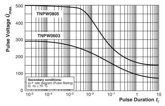
Maximum pulse voltage, single and continuous pulses; applicable if  $P \leq P_{\text{max}}$ ; for permissible resistance change equivalent to 8000 h operation in standard operation mode
