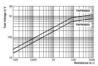
Single-Pulse High Voltage Overload Test 1.2/50 µs EN 140000 4.27
