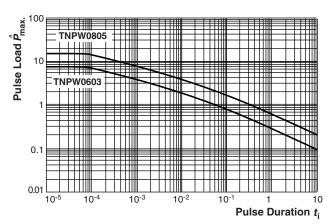
Maximum pulse load, single pulse; applicable if  $\bar{P} \to 0$  and  $n \le 1000$  and  $\hat{U} \le \hat{U}_{max}$ ; for permissible resistance change equivalent to 8000 h operation in standard operation mode
