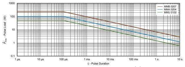
Maximum pulse load, single pulse; applicable if  $\bar{P} \to 0$  and n  $\leq 1000$  and  $\hat{U} \leq \hat{U}_{\max}$ ; for permissible resistance change  $\pm (0.5~\%~R + 0.01~\Omega)$
