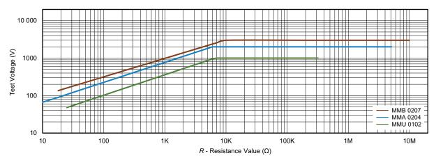
Pulse load rating in accordance with IEC 60115-1 clause 4.27; 1.2 µs/50 µs; 5 pulses at 12 s intervals; for permissible resistance change  $\pm$  (0.5 % R + 0.05  $\Omega)$
