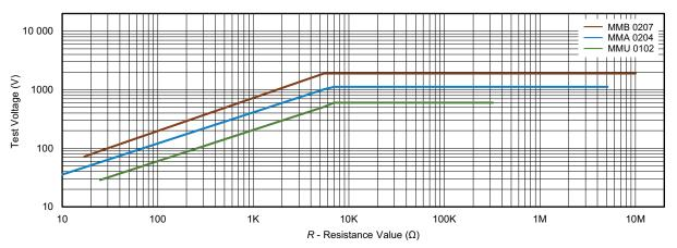
Pulse load rating in accordance with IEC 60115-1 clause 4.27; 10  $\mu$ s/700  $\mu$ s; 10 pulses at 1 minute intervals; for permissible resistance change  $\pm$  (0.5 % R + 0.05  $\Omega$ )
