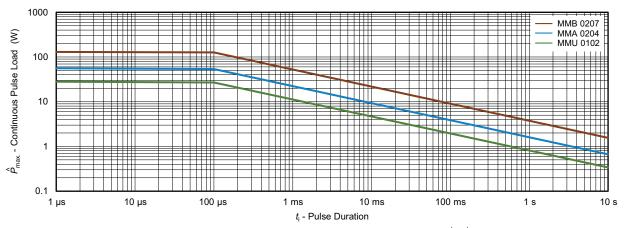
Maximum pulse load, continuous pulse; applicable if  $\bar{P} \leq P\left(\vartheta_{\rm amb}\right)$  and  $\hat{U} \leq \hat{U}_{\rm max}$ ; for permissible resistance change  $\pm$  (0.5 % R + 0.01  $\Omega$ )
