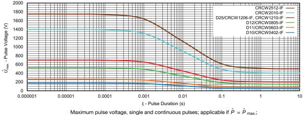
Maximum pulse voltage, single and continuous pulses; applicable if  $P = P_{max}$ ; for permissible resistance change equivalent to 8000 h operation
