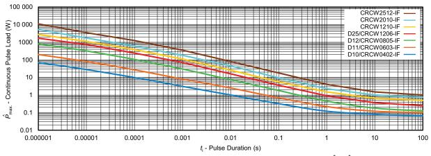
Maximum pulse load, continuous pulses; applicable if  $\overline{P} \le P(v_{amb})$  and  $\hat{U} = \hat{U}_{max}$ ; for permissible resistance change equivalent to 8000 h operation
