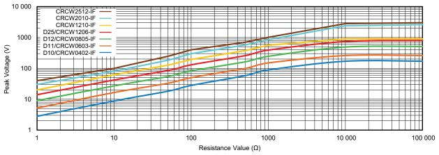
Pulse load rating in accordance to EN 60115-1, 4.27; 10 µs / 700 µs; 10 pulses at 1 min intervals; for permissible resistance change 1 %
