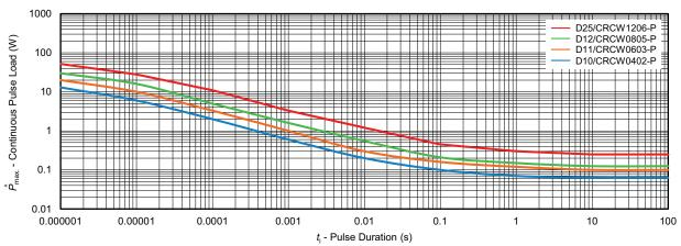
Maximum pulse load, continuous pulses; applicable if  $\overline{P} \le P$  ( $\vartheta_{amb}$ ) and  $\hat{U} = \hat{U}_{max}$ ; for permissible resistance change equivalent to 8000 h operation
