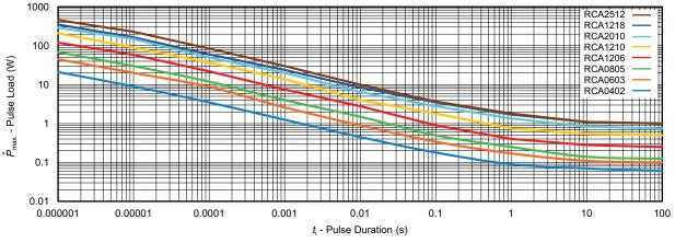
Maximum pulse load, single pulse; applicable if  $\overline{P} \rightarrow 0$  and n < 1000 and  $\hat{U} = \hat{U}_{max}$ ; for permissible resistance change equivalent to 8000 h operation
