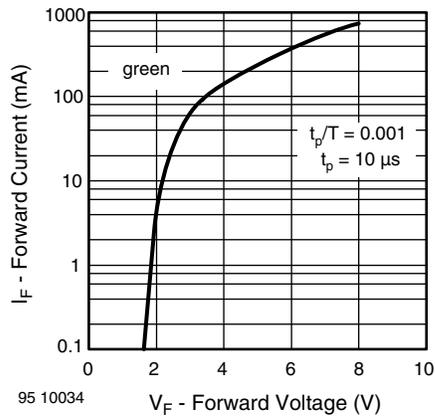
Fig. 15 - Forward Current vs. Forward Voltage
