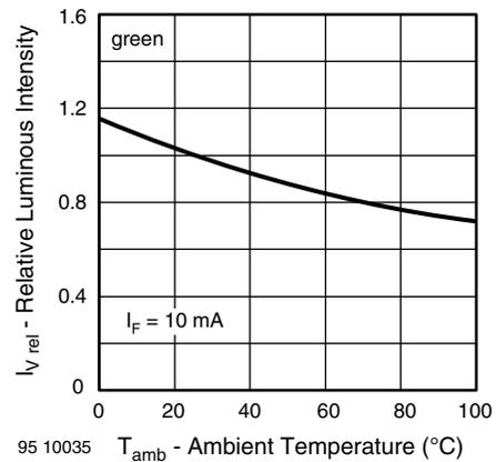
Fig. 18 - Relative Luminous Intensity vs. Ambient Temperature
