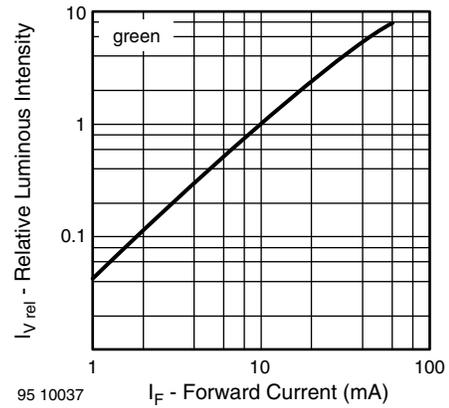
Fig. 16 - Relative Luminous Intensity vs. Forward Current
