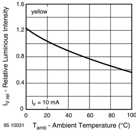
Fig. 13 - Relative Luminous Intensity vs. Ambient Temperature
