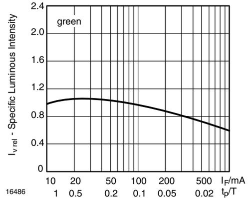
Fig. 17 - Relative Luminous Intensity vs. Forward Current/Duty Cycle
