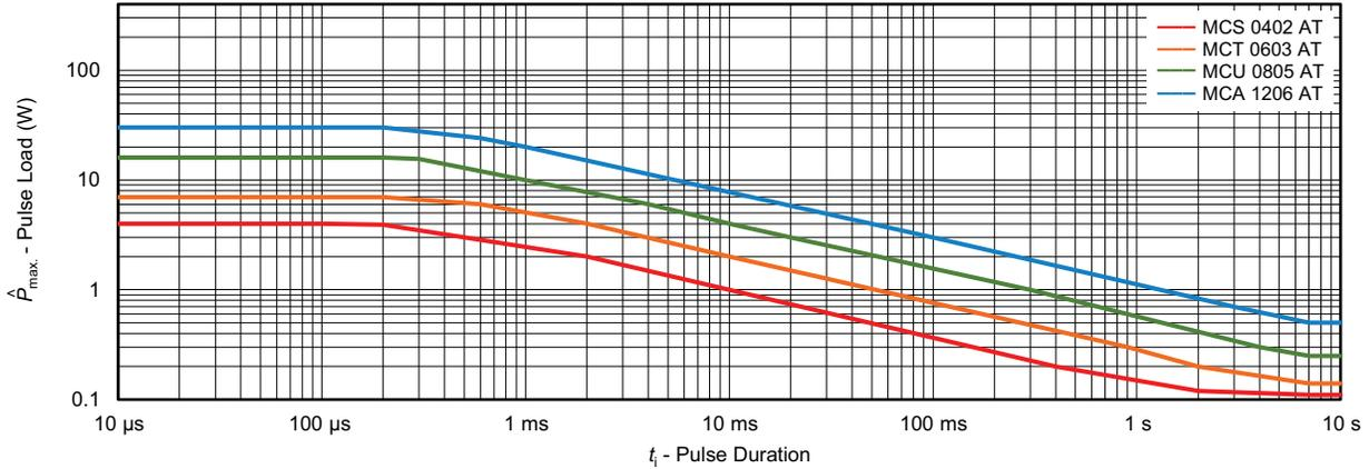
Maximum pulse load, single pulse; applicable if  $\bar{P} \rightarrow 0$  and  $n \leq 1000$  and  $\hat{U} \leq \hat{U}_{max}$ ; for permissible resistance change equivalent to 8000 h operation in standard operation mode
