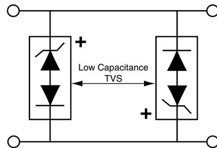
**Application Note:** Device must be used with two units in parallel, opposite in polarity as shown in circuit for AC signal line protection.
