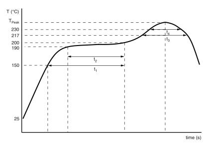
Fig. 4 - Maximum temperature load during reflow soldering
