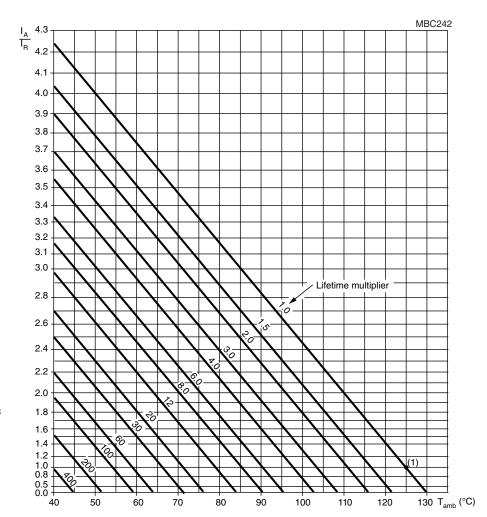
$I_{\rm A}$  = Actual ripple current at 100 kHz  $I_{\rm R}$  = Rated ripple current at 100 kHz, 125 °C  $^{(1)}$  Useful life at 125 °C and  $I_{\rm R}$  applied; see Table 7
