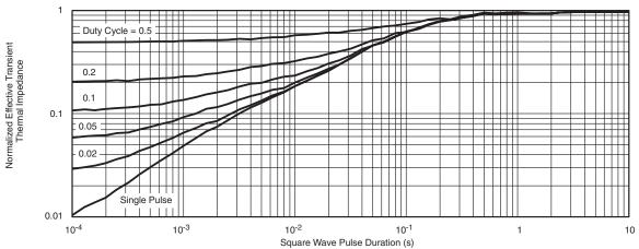
Normalized Thermal Transient Impedance, Junction-to-Foot
