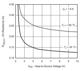
On-Resistance vs. Gate-to-Source Voltage
