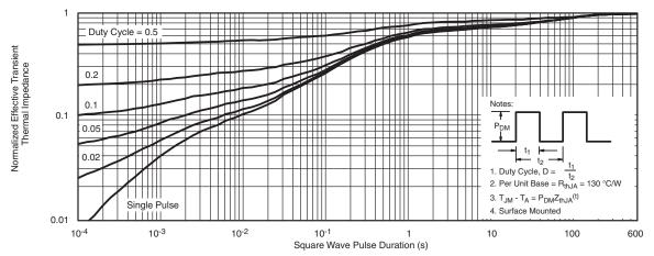
Normalized Thermal Transient Impedance, Junction-to-Ambient
