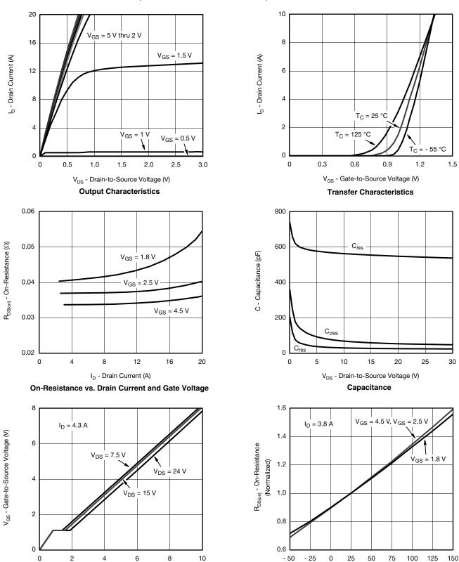
$\mathbf{Q}_{\mathbf{g}}$  - Total Gate Charge (nC)  $\mathbf{Gate} \ \mathbf{Charge}$  T<sub>J</sub> - Junction Temperature (°C)
