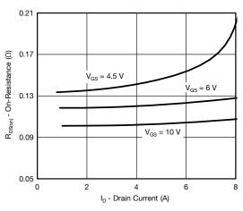
On-Resistance vs. Drain Current and Gate Voltage
