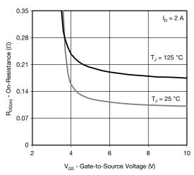
On-Resistance vs. Gate-to-Source Voltage
