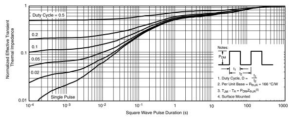
Normalized Thermal Transient Impedance, Junction-to-Ambient
