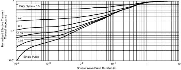
Normalized Thermal Transient Impedance, Junction-to-Foot
