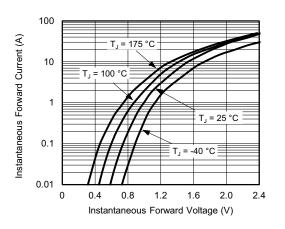
Fig. 3 - Typical Instantaneous Forward Characteristics
