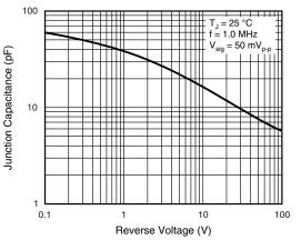
Fig. 5 - Typical Junction Capacitance
