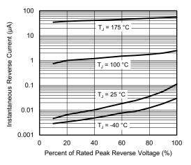
Fig. 4 - Typical Reverse Leakage Characteristics
