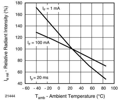
Fig. 6 - Relative Radiant Intensity vs. Ambient Temperature
