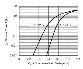
**Source Drain Diode Forward Voltage**
