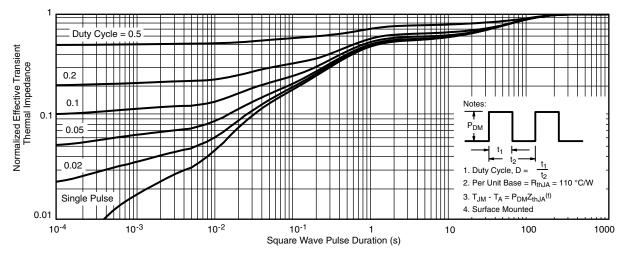
Normalized Thermal Transient Impedance, Junction-to-Ambient
