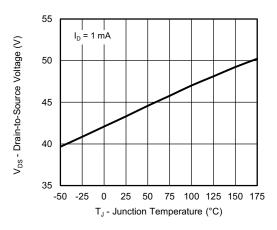
**Drain Source Breakdown vs. Junction Temperature**
