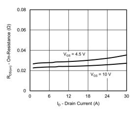
On-Resistance vs. Drain Current
