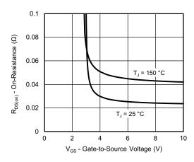
On-Resistance vs. Gate-to-Source Voltage
