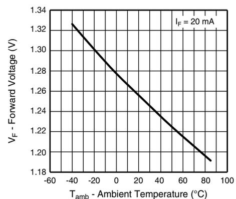
Fig. 4 - Forward Voltage vs. Ambient Temperature
