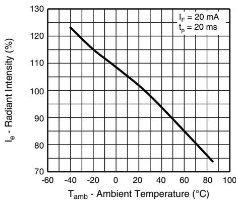
Fig. 7 - Relative Radiant Intensity vs. Ambient Temperature
