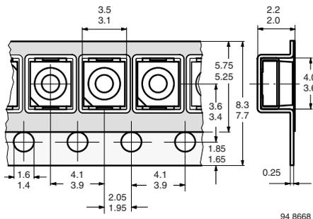
Fig. 9 - Tape Dimensions in mm for PLCC-2
