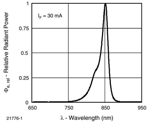
Fig. 5 - Relative Radiant Power vs. Wavelength
