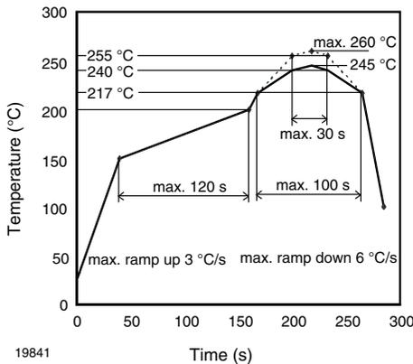
Fig. 7 - Lead (Pb)-free Reflow Solder Profile acc. J-STD-020
