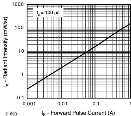
Fig. 4 - Radiant Intensity vs. Forward Current
