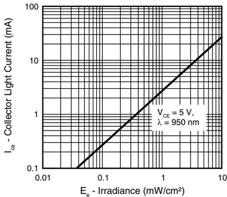
Fig. 3 - Collector Light Current vs. Irradiance
