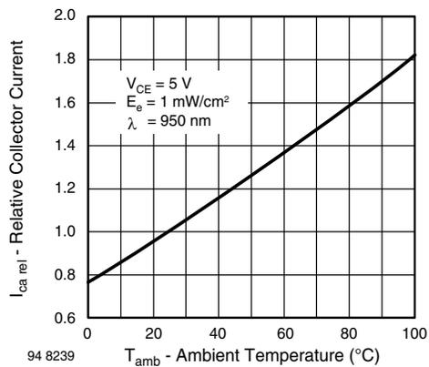
Fig. 7 - Relative Collector Current vs. Ambient Temperature
