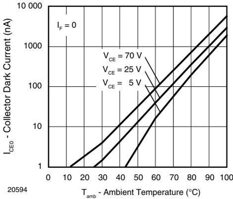
Fig. 2 - Collector Dark Current vs. Ambient Temperature
