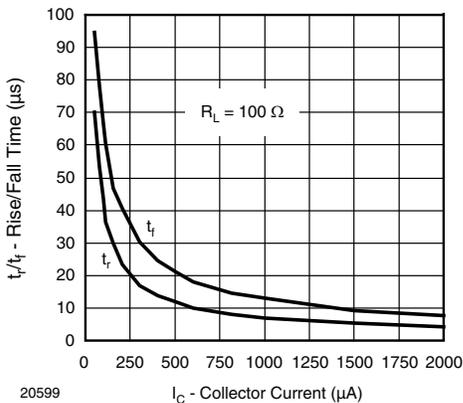
Fig. 4 - Rise/Fall Time vs. Collector Current
