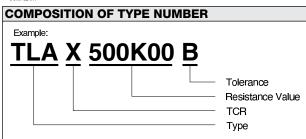
Resistance value, in ohm, is expressed by a series of six characters, five of which represent significant digits. K or M is a dual-purpose letter that designates both the value range (K for kilo-ohm; M for mega-ohm) and the location of decimal point.
