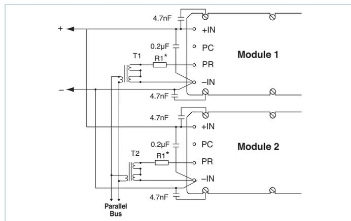
Figure 10 — Transformer-coupled interface
