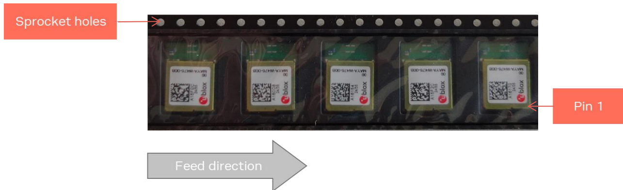
Figure 17: Orientation of MAYA-W4 modules on tape
