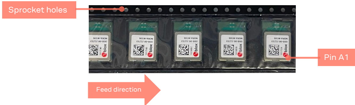
Figure 7: NORA-W306 module on tape orientation
