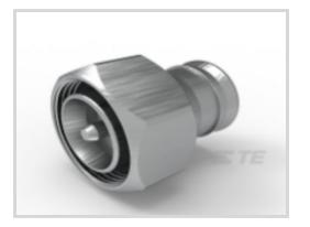
RF Interface: **4.3-10** RF Connector Style: **Plug** RF Connector Mated Outer Diameter (Approximate): **25 mm [.984 in ]** Impedance: **50 Ω** Compatible With RF Cable Type: **1/2" Flex Cable**
