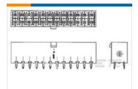
TE Part #1-1586038-0 10P VRT HDR VAL-U-LOK V0
