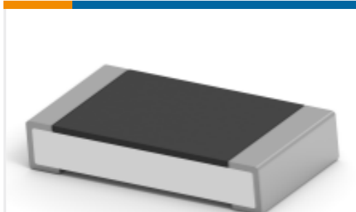
TE Part #2-2176390-6 RQ 1206 2K1 0.1% 10PPM 5K RL
