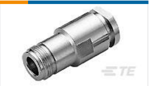
TE Part #1-1337406-0 N Str Jk PS 50Ohm Silver Pltd PSF 1/4M,
