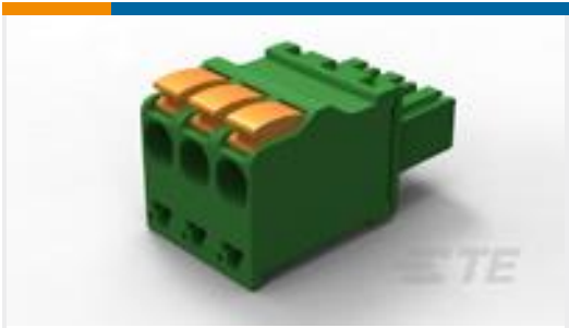
TE Part #1986720-3 STR PLUG SPRING TYPE RH 3P, 3.81mm
