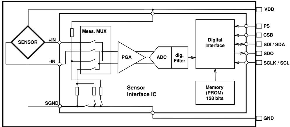
Figure 1: Block diagram of MS5803-07BA
