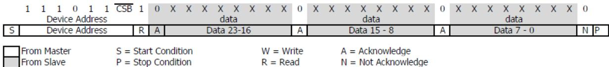
Figure 6: I<sup>2</sup>C pressure response (D1) on 24 bit from MS5803-07BA
