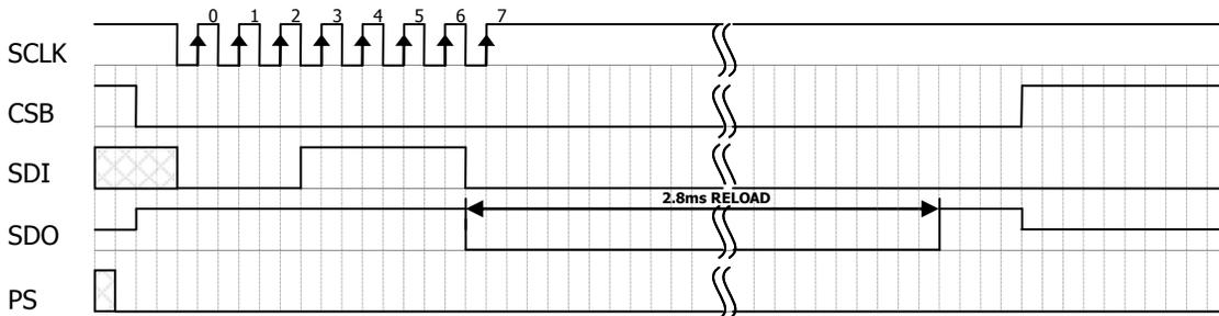
Figure 10: Reset command sequence SPI mode 3
