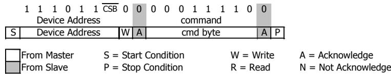
Figure 3: I<sup>2</sup>C Reset Command
