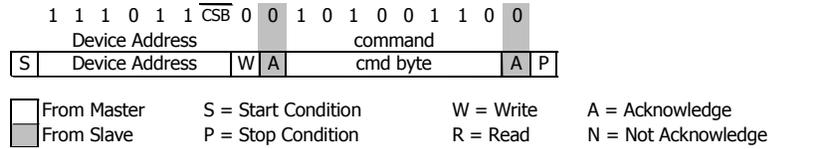
Figure 7: I<sup>2</sup>C Command to read memory address= 011 (Coefficient 3)
