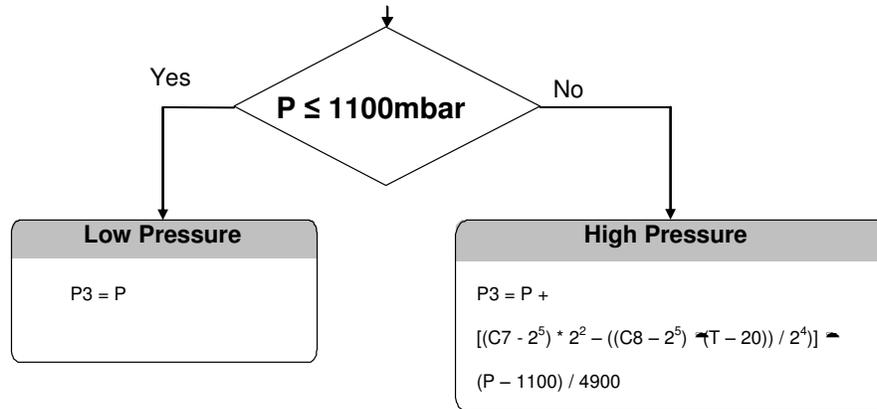
Figure 18: Flow chart for High pressure P3 calculation
