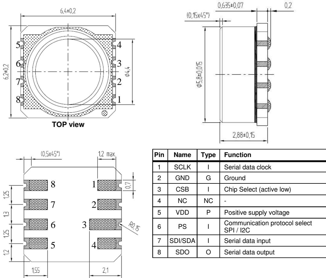
Figure 20: MS5803-07BA package outlines, pin configuration and description
