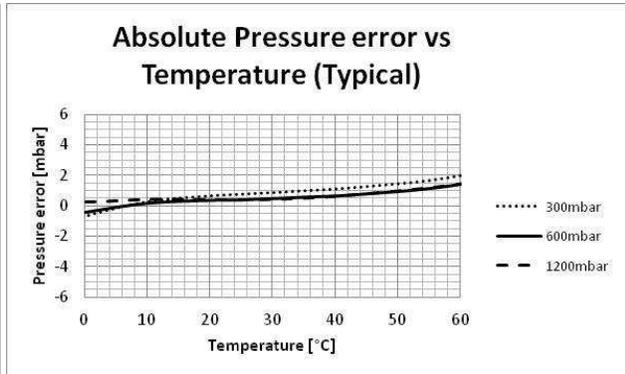
TEMPERATURE ERROR VS TEMPERATURE AND PRESSURE
