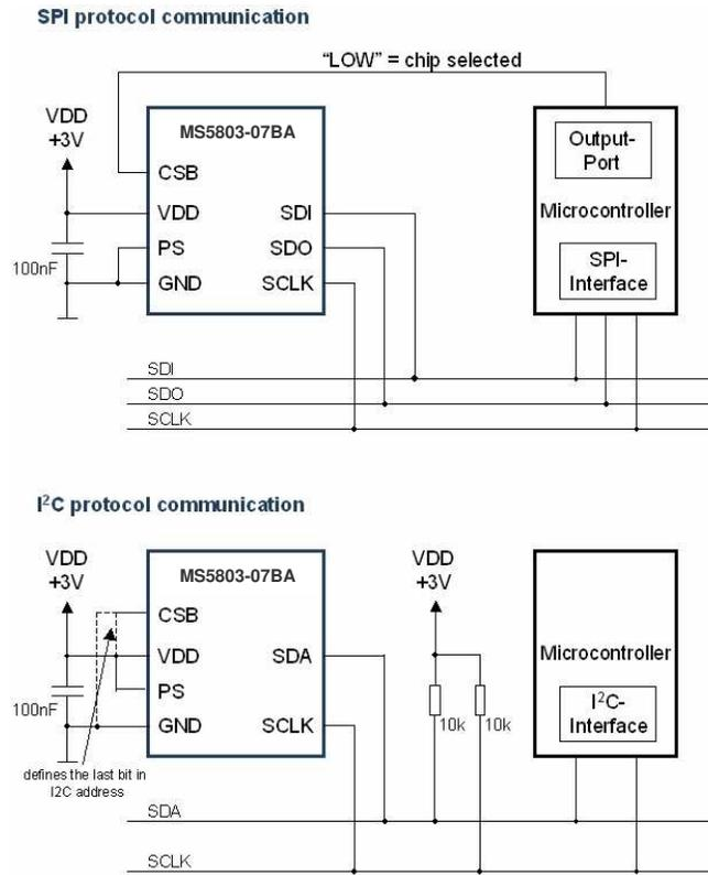
Figure 19: Typical application circuit with SPI / I<sup>2</sup>C protocol communication
