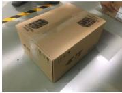
After Test: Carton was OK. Inner packaging was OK. Parts were Ok.
