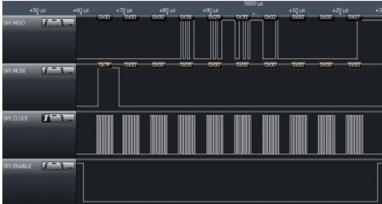
Figure 5-23. Continuous Read of FIFO After Inventory Command
