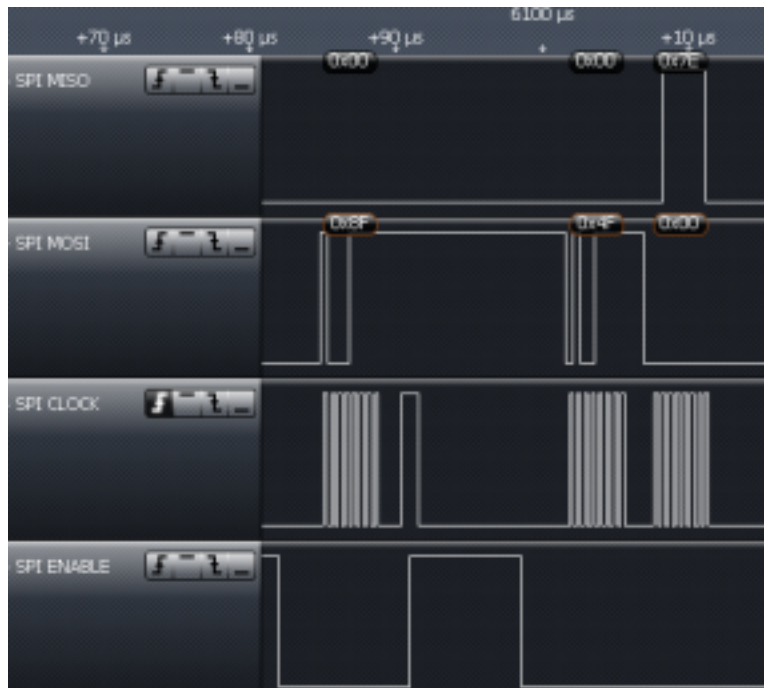
Figure 5-25. Reset FIFO and Read RSSI
