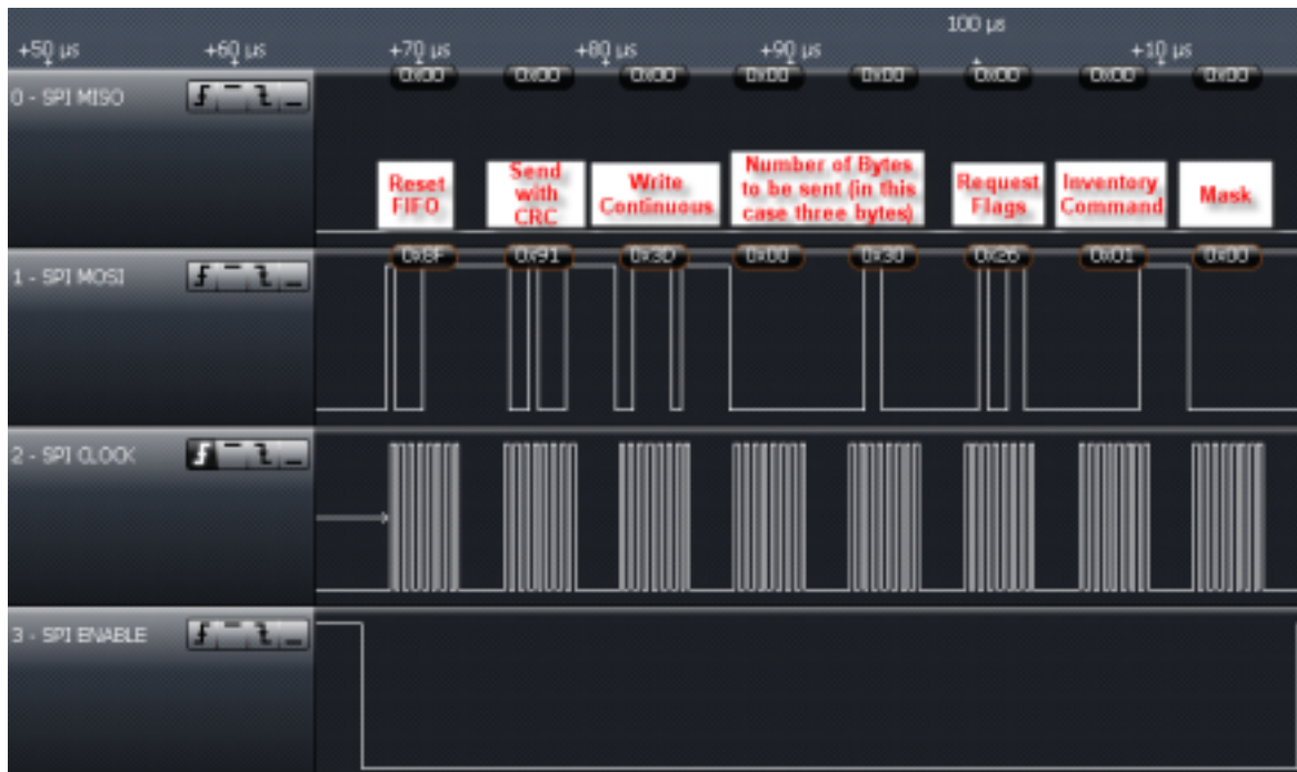
Figure 5-20. Inventory Command Sent From MCU to TRF7970A
