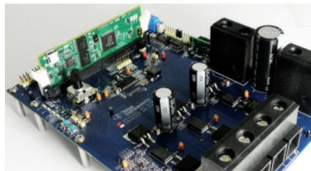
Three Phase BLDC & PMSM Motor Kit with DRV8302 and Piccolo MCU - DRV8302-HC-C2-KIT
