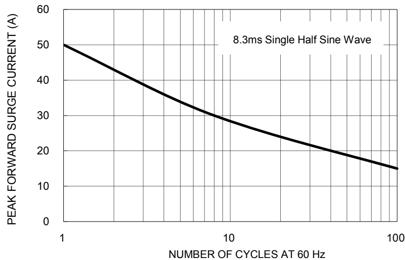
FIG. 3 MAXIMUM NON-REPETITIVE PEAK FORWARD SURGE CURRENT
