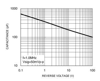
Fig.2 Typical Junction Capacitance
