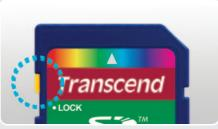
Mechanical write-protection switch
