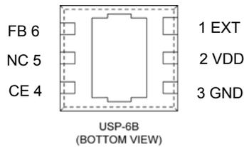
The dissipation pad for the USP-6B package should be solder-plated in recommended mount pattern and metal masking so as to enhance mounting strength and heat release.
