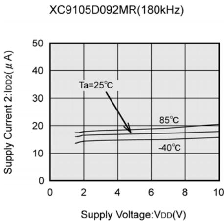
(7) Stand-By Current vs. Power Supply Voltage
