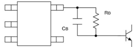
Insert  $R_B$  and  $C_B$  when using a bipolar NPN Transistor.
