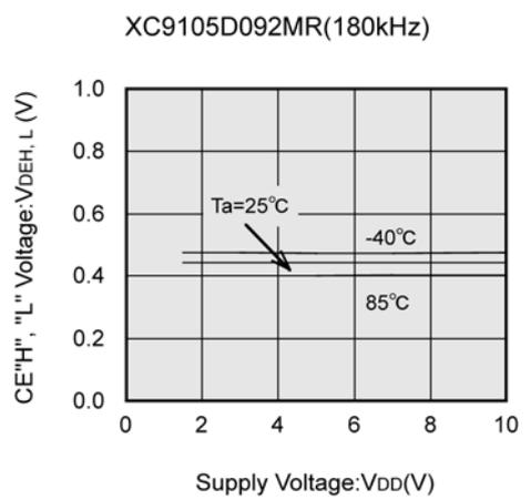
(14) PWM "H" "L" Voltage vs. Power Supply Voltage
