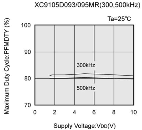
(24) PFM Duty Ratio vs. Power Supply Voltage
