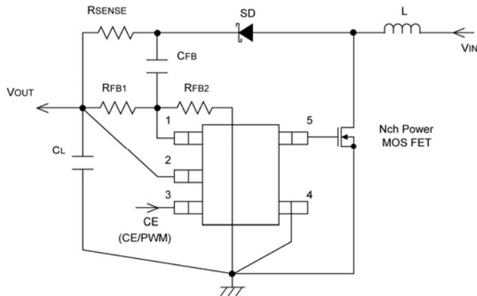
When obtaining  $V_{DD}$  from a source other than  $V_{OUT}$ , please insert a capacitor  $C_{DD}$  between the  $V_{DD}$  pin and the GND pin in order to provide stable operations. Please place  $C_L$  and  $C_{DD}$  as close as to the  $V_{OUT}$  and  $V_{DD}$  pins respectively and also close to the GND pin. Strengthen the wiring sufficiently.  $R_{SENSE}$  should be removed and shorted when the  $C_L$  capacitor except for ceramic or low ESR capacitor is used.
