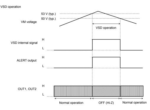
Note: The VSD circuit is activated if the absolute maximum voltage rating is violated. Note that the circuit is provided as an auxiliary only and does not necessarily provide the IC with a perfect protection from any kind of damages.
