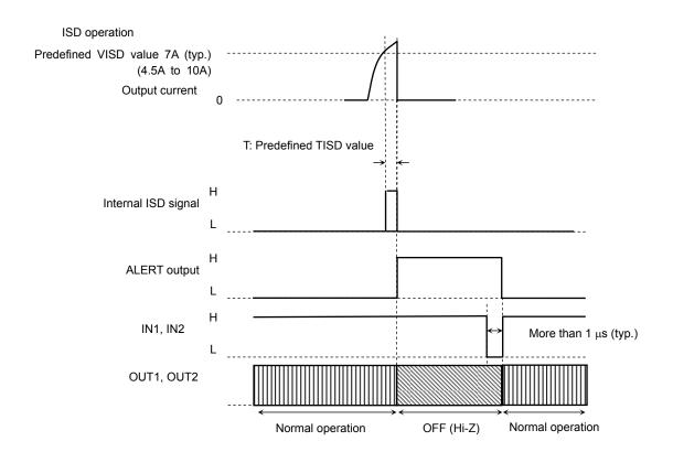
Note: The ISD circuit is activated if the absolute maximum current rating is violated. Note that the circuit is provided as an auxiliary only and does not necessarily provide the IC with a perfect protection from damages due to overcurrent caused by power fault, ground fault, load-short and the like.
