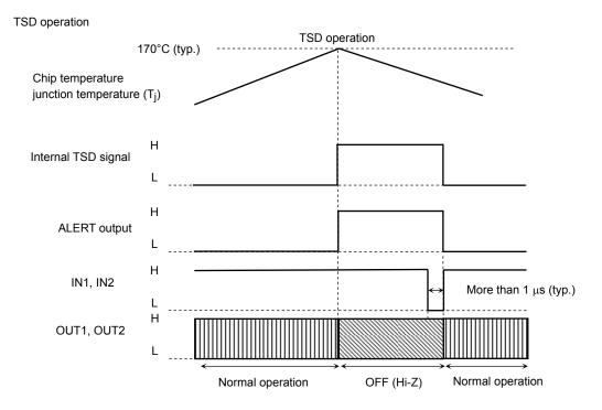
Note: The TSD circuit is activated if the absolute maximum junction temperature rating (T<sub>j</sub>) of 150°C is violated. Note that the circuit is provided as an auxiliary only and does not necessarily provide the IC with a perfect protection from any kind of damages.
