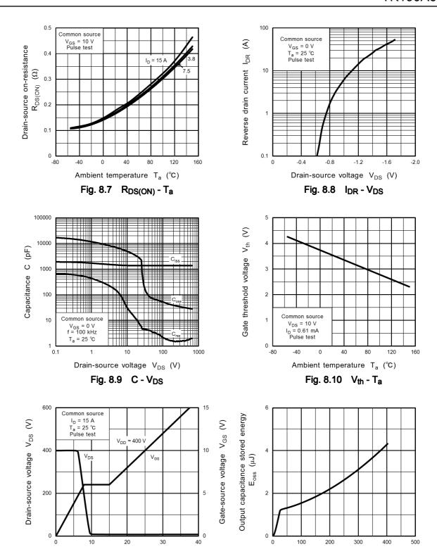
Drain-source voltage  $V_{DS}$  (V) Fig. 8.12 E<sub>OSS</sub> - V<sub>DS</sub>
