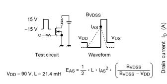
Fig. 8.16 Test Circuit/Waveform
