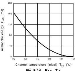
Fig. 8.14 E<sub>AS</sub> - T<sub>ch</sub> (Guaranteed Maximum)
