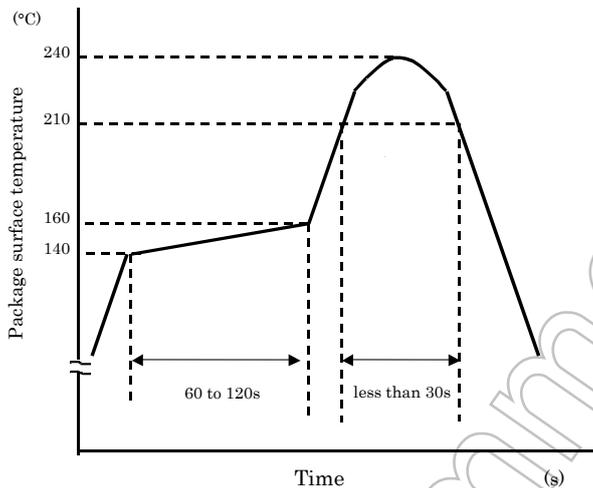
This profile is based on the device's maximum heat resistance guaranteed value. Set the preheat temperature/heating temperature to the optimum temperature corresponding to the solder paste type used by the customer within the described profile.
